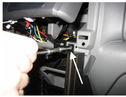
Attach upper portion of console to dash using screws that held top of lower trim panel
